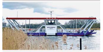
Year of manufacture 2023 Length 34 m | Width 9 m Drive: DST2 electric motor Battery and solar support
