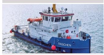
Year of manufacture 2019 Length 22 m | Width 7.5 m Work ship with diesel-electric drive system, 2x drive units DST2 225 kW
