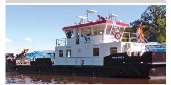
Year of manufacture 2020 Length 38 m | Width 8.0 m WSA work ship with diesel-electric drive system 2x diesel Scania, 2x drive units DST2 225 kW
