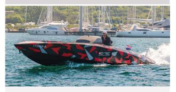
Year of manufacture 2022 Length 9 m | Width 2.50 m | Maximum speed 40 kn Drives: 2x 200 kW, controllers: b maXX mobil Battery capacity: 98 kWh
