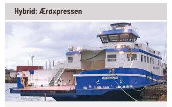
Year of manufacture 2019 Length 49.36 m | Width 12.50 m | Draft 1.92 m Drives: 2x Scania DI16 8-cylinder diesel motors, 2x drive units 450 kW
