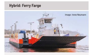
Year of manufacture 2017 Length 59 m | Width 14 m | Maximum speed 14 km/h Capacity: 32-34 passenger cars, 6 semis, up to 249 people Drives: 4x DS2 main motors 200 kW each
