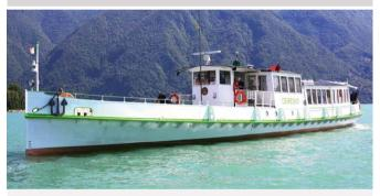
Year of manufacture 2021 Length 31.35 m | Width 6.28 m Drives: 2x DST2-260 electric motor 180 kW Battery capacity: 840 kWh, charging station: 1.6 MW charger
