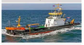
Year of manufacture 2022 Length 48 m | Width 12 m Water injection dredger with diesel-electric drive system 5x diesel generators, 2x rudder propellers 450 kW
