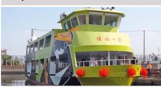
Year of manufacture 2017 Length 25 m | Width 6.5 m Capacity: up to 150 persons; 46 bicycles Drives: 2x 2 powerMELA® systems, each with 150 kW
