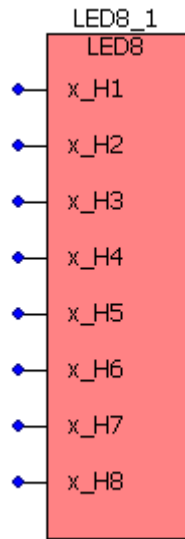
Figure 35: LED8 function block for BMC-M-PLC-01
