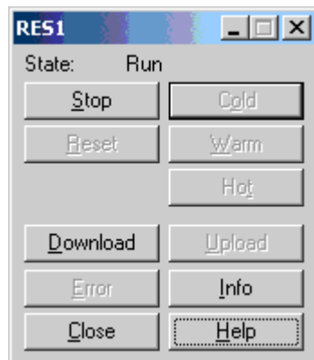
Figure 20: Functions of the control dialog of the selected resource in the "RUN" status.
