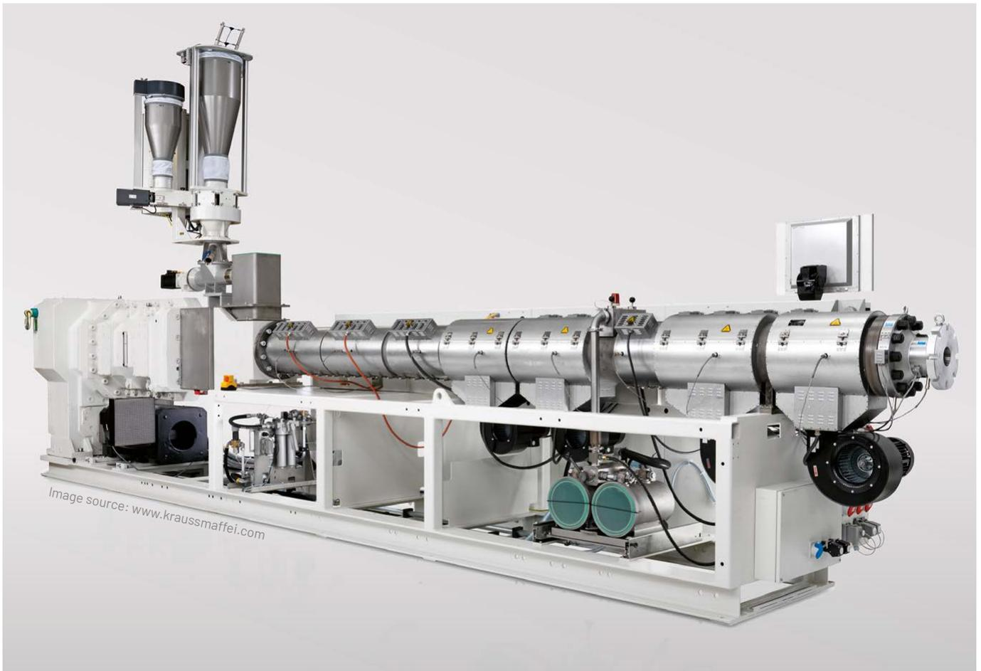
Baumüller offers energy-efficient direct drive technology for extrusion machines. With this technology you can minimize drive losses, reduce background noise during operation and increase the reliability of the machines. At the same time, the lack of gearing means a smaller size for the machines, which can be designed more compactly.
