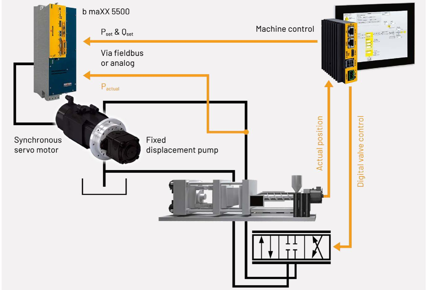
The servo-hydraulic system consists of a servo drive, which drives a synchronous servo motor. This motor drives a fixed displacement pump. The pressure and volume flow set values ( $P_{set}$  and  $Q_{set}$ ) are sent from the control unit to the servo drive. Pressure and flow rate are controlled on the servo drive by adjusting the speed. As in the conventional hydraulic systems with standard motors, the actual positions are read out via the machine control unit.
