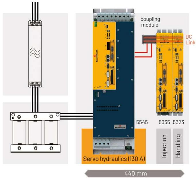
All drive solutions are compact and scalable, and allow high power density. Due to the identical controller firmware, costs for project planning, maintenance, and service are also reduced.
