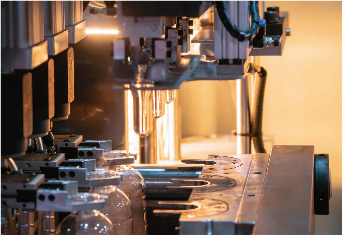
The drive concepts from Baumüller are the optimal solution for reducing energy requirements in blow molding machines. Water-cooled motors and converters in particular succeed with their highly compact design and rapid heat dissipation.
