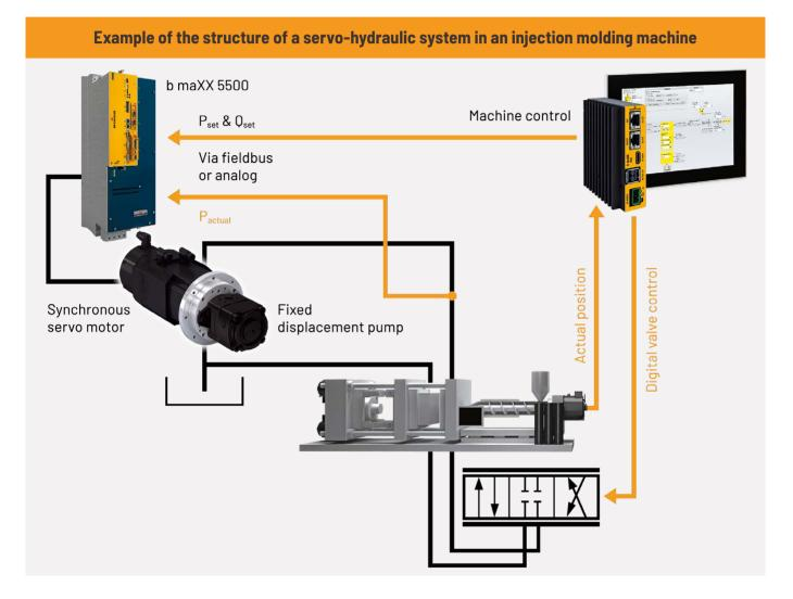
The servo-hydraulic system consists of a servo drive, which drives a synchronous servo motor. This motor drives a fixed displacement pump. The pressure and volume flow set values (Pset and Qset) are sent from the control unit to the servo drive. Pressure and flow rate are controlled on the servo drive by adjusting the speed. As in the conventional hydraulic systems with standard motors, the actual positions are read out via the machine control unit.
