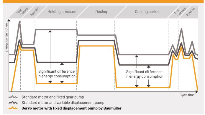
The difference in energy consumption can be clearly seen in the typical hydraulic system shown in the diagram. The high energy efficiency of the servo-hydraulic solution arises from a needs-specific pump output. When the machine is at rest, e.g. during cooling, then the motors will also be at rest and will consume no energy.
