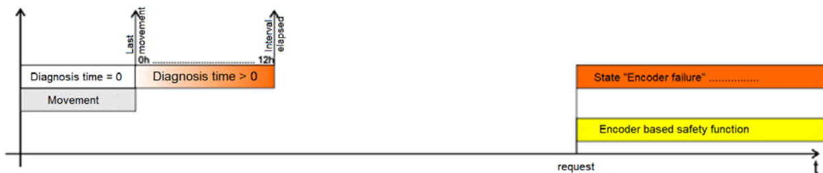
Figure 4: Encoder monitoring at the SINCOS encoder with asynchronous motor Diagnosis time of 12 h expired -> the safety function is requested once more
