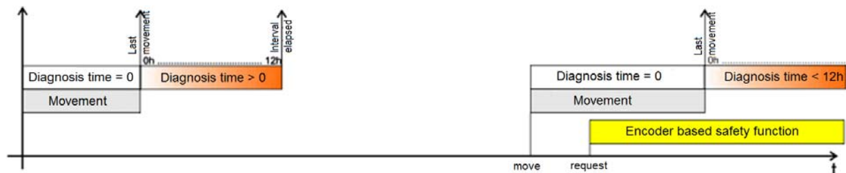
Figure 8: Encoder monitoring of the SINCOS encoder with asynchronous motor Expiration of diagnostic time -> Movement -> Demand
