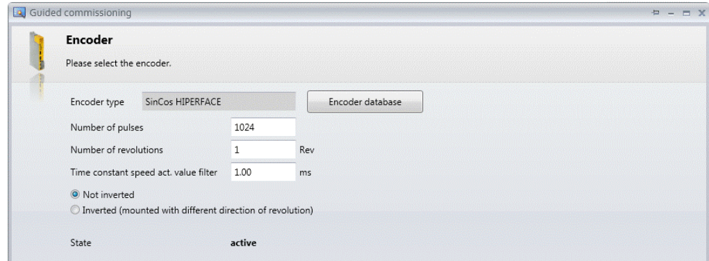
Figure 32: Guided commissioning: Selecting the encoder
