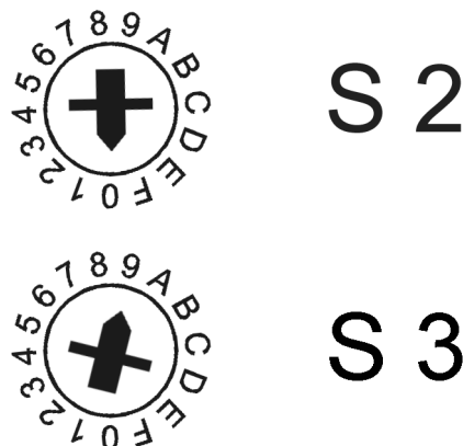
Figure 15: Example: Set the Ethernet address 192.168.1.10 (rotary switch S2 on 0 and rotary switch S3 on 9)
