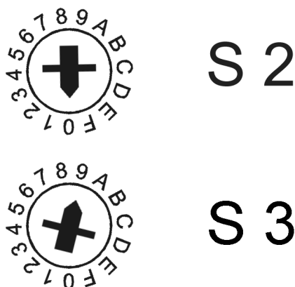
Figure 20: Example: Set the Ethernet address 192.168.1.10 (rotary switch S2 to 0, rotary switch S3 to 9)
