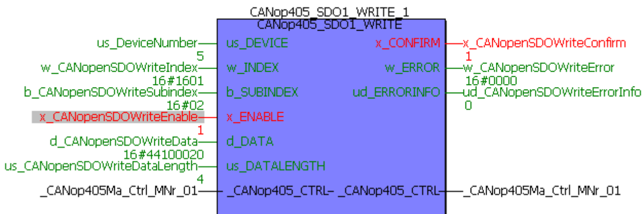
Figure 91: Entering second mapped object of second receive PDO
