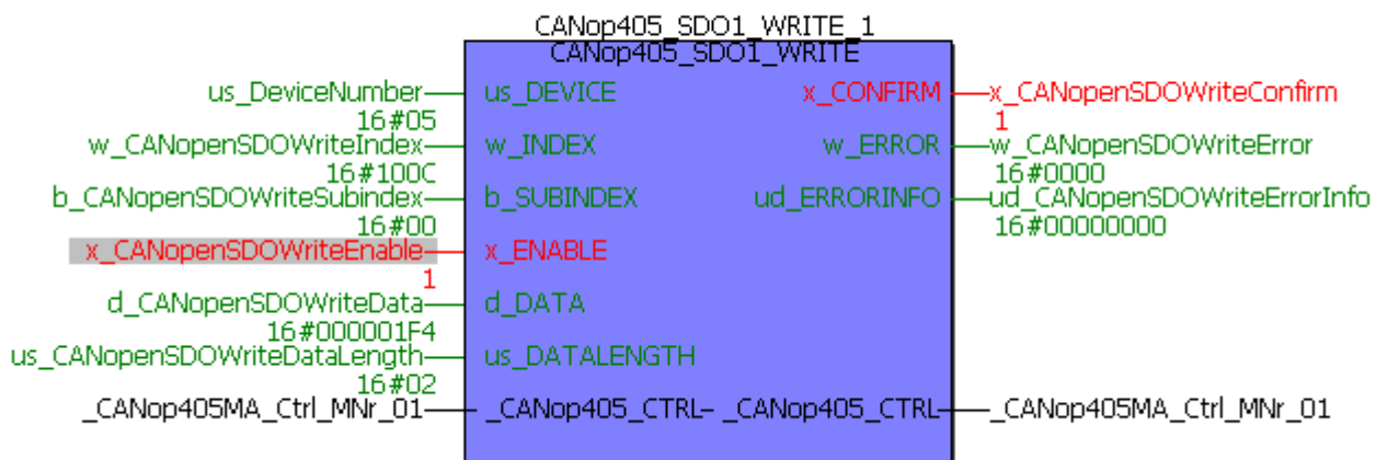
Figure 112: Setting Node Guarding Time on CANopen slave
