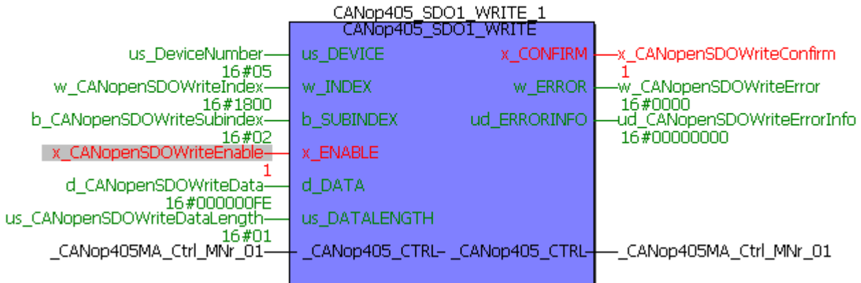
Figure 103: Writing configuration of first transmit PDO of CANopen slave - Subindex 2
