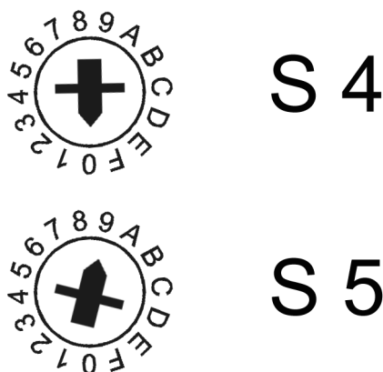
Figure 16: Example: Set the Ethernet address 192.168.1.10 (rotary switch S4 to 0, rotary switch S5 to 9)
