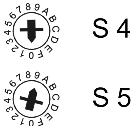
Figure 11: Example: Set the Ethernet address 192.168.1.10 (rotary switch S4 on 0 and rotary switch S5 on 9)
