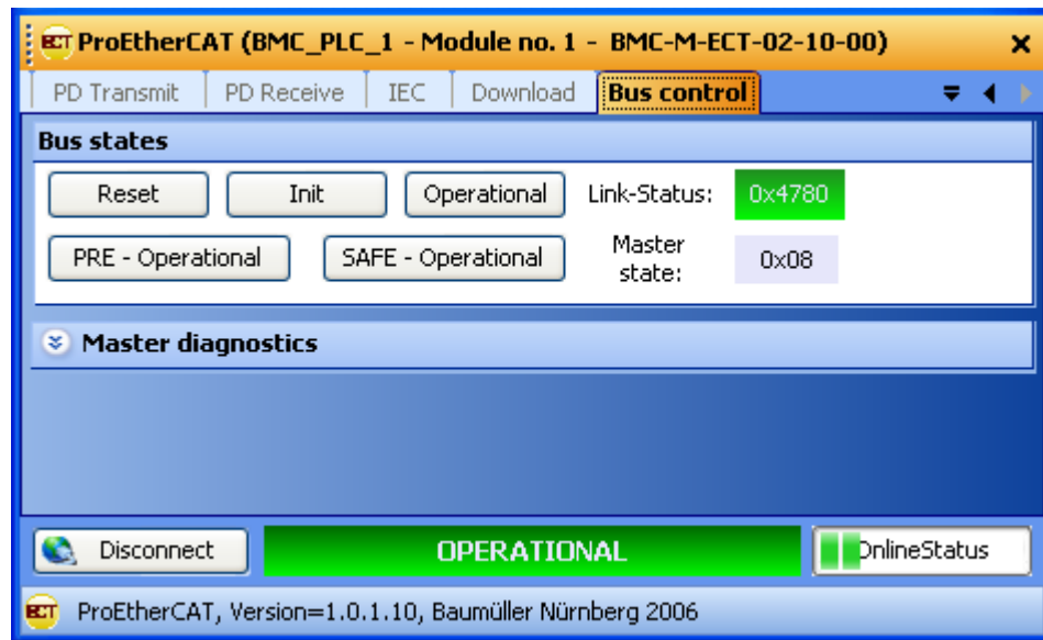
Figure 54: ProEtherCAT - EtherCAT master communication configuration, "Bus Control" tab
