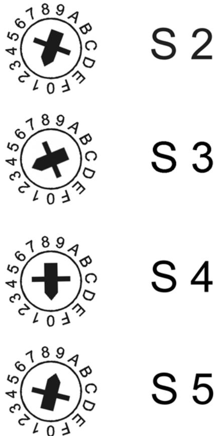
Figure 28: Example: Setting of the Ethernet-address 192.168.20.10
