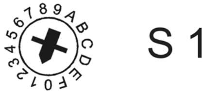
Figure 16: Example: Setting of the module address 1 (switch S1 to 1)
