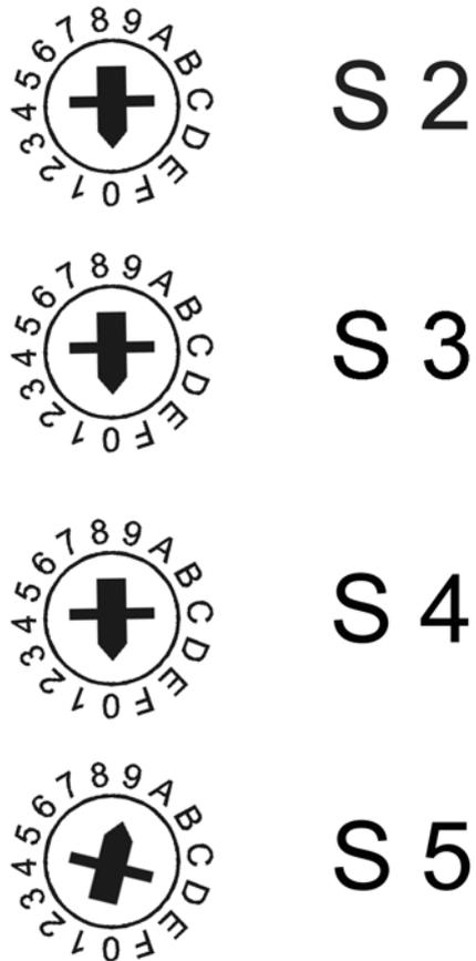
Figure 17: Example: Setting of the coding value 16H0009
