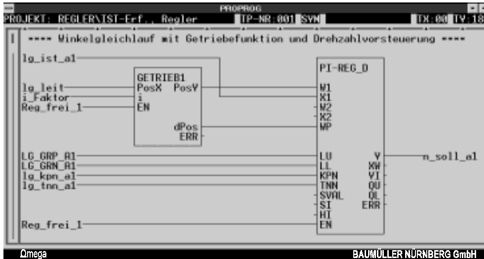
Figure 1.3: Sample program: Accurate synchronism with gear function and speed control
