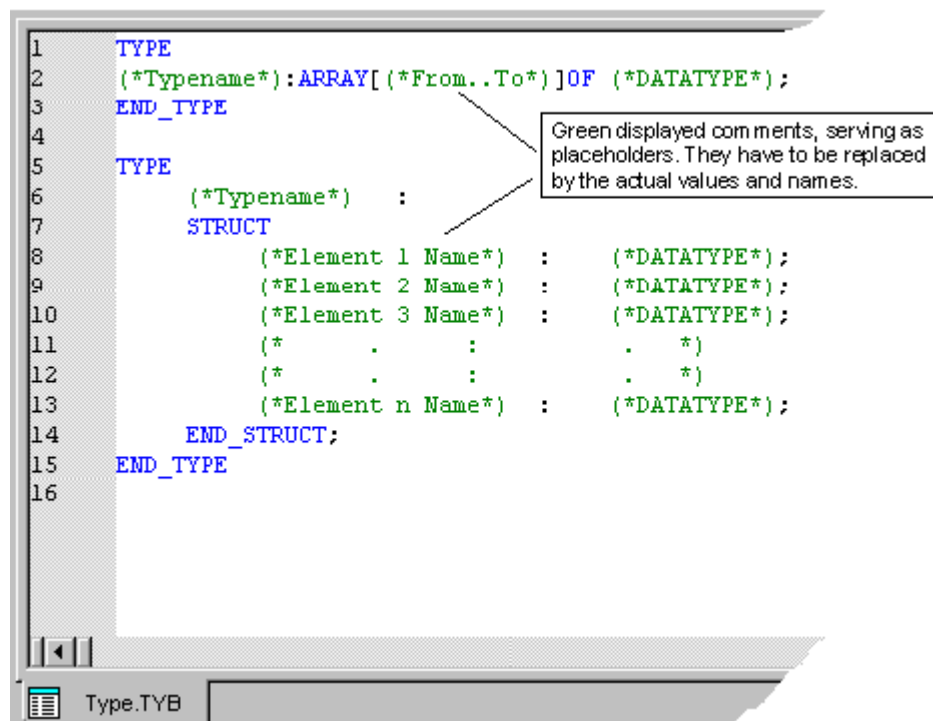
Figure 56: Data type worksheet 'Type' with pre-edited keywords, inserted using the Edit Wizard
