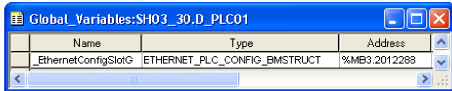
Figure 18: Example: Global variable of type ETHERNET_PLC_CONFIG_BMSTRUCT (ProProg wt III)
