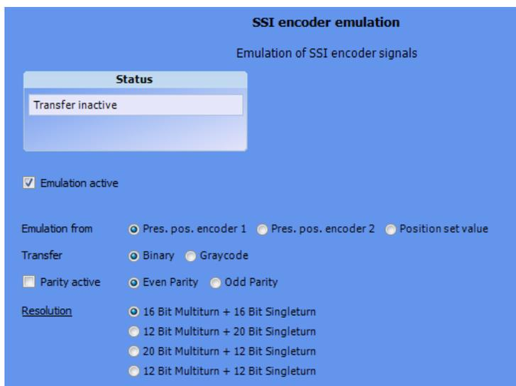
Figure 20: Settings SSI encoder emulation
