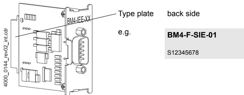
Figure 11: Type plate **BM4-F-SIE-XX** for standard controller
