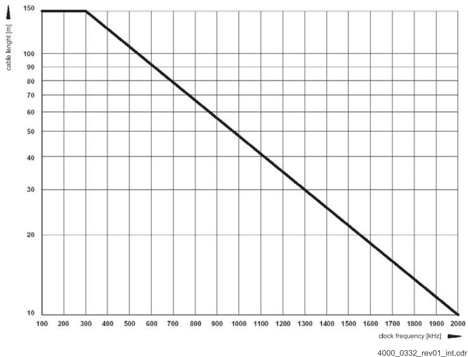
Figure 15: Cable length SSI encoder emulation
