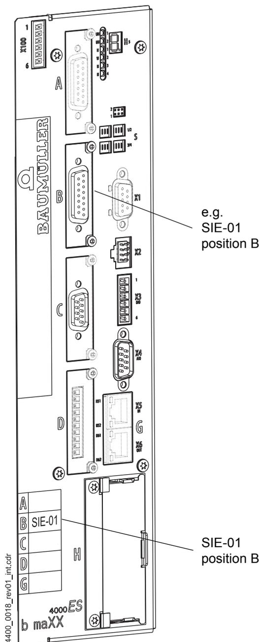
Figure 12: SSI encoder emulation in ES controller
