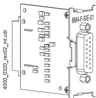
Figure 13: BM4-F-SIE-XX for standard controller
