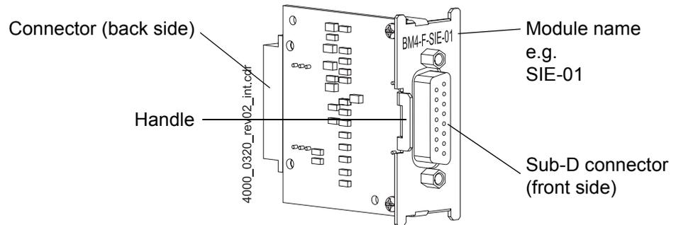
Figure 10: **BM4-F-SIE-XX** for standard controller
