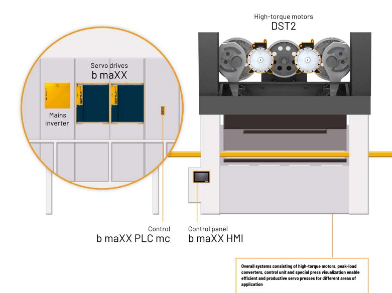
The drive system is linked to a higher-level control system via a predefined interface and is vendor-neutral. Our DST2 series high-torque motors achieve very high maximum torques, in order to provide the necessary power for the forming process. The motors can be perfectly adapted to the press's requirements thanks to different shaft and flange options. We also enable the press power to be divided between multiple motors connected via a master-slave coupling.
