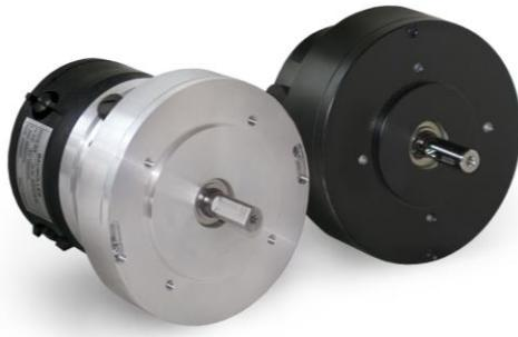
The Baumüller direct current – disc motors are permanent magnet excited motor with ironless rotor and drum-shaped commutator, thus low inertia and highly dynamic running characteristics. They can be easily controlled over their entire speed range and even at the lowest speeds, less than one revolution per minute, the concentricity is maintained exactly.
